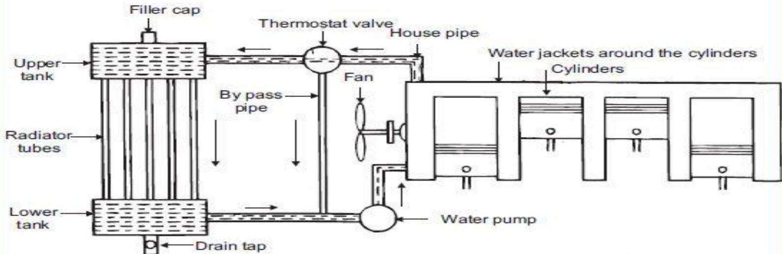
**Figure 5.5 : Water Cooling System of a 4-cylinder Engine**
