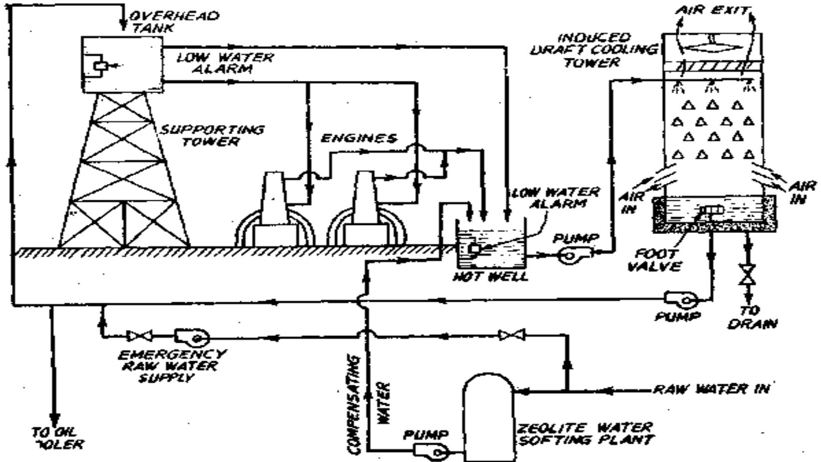
Fig. 23.3. Cooling water system using water softening plant and cooling-tower.
