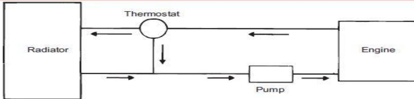
**Figure 5.4 : Water Cooling System using Thermostat Valve**
