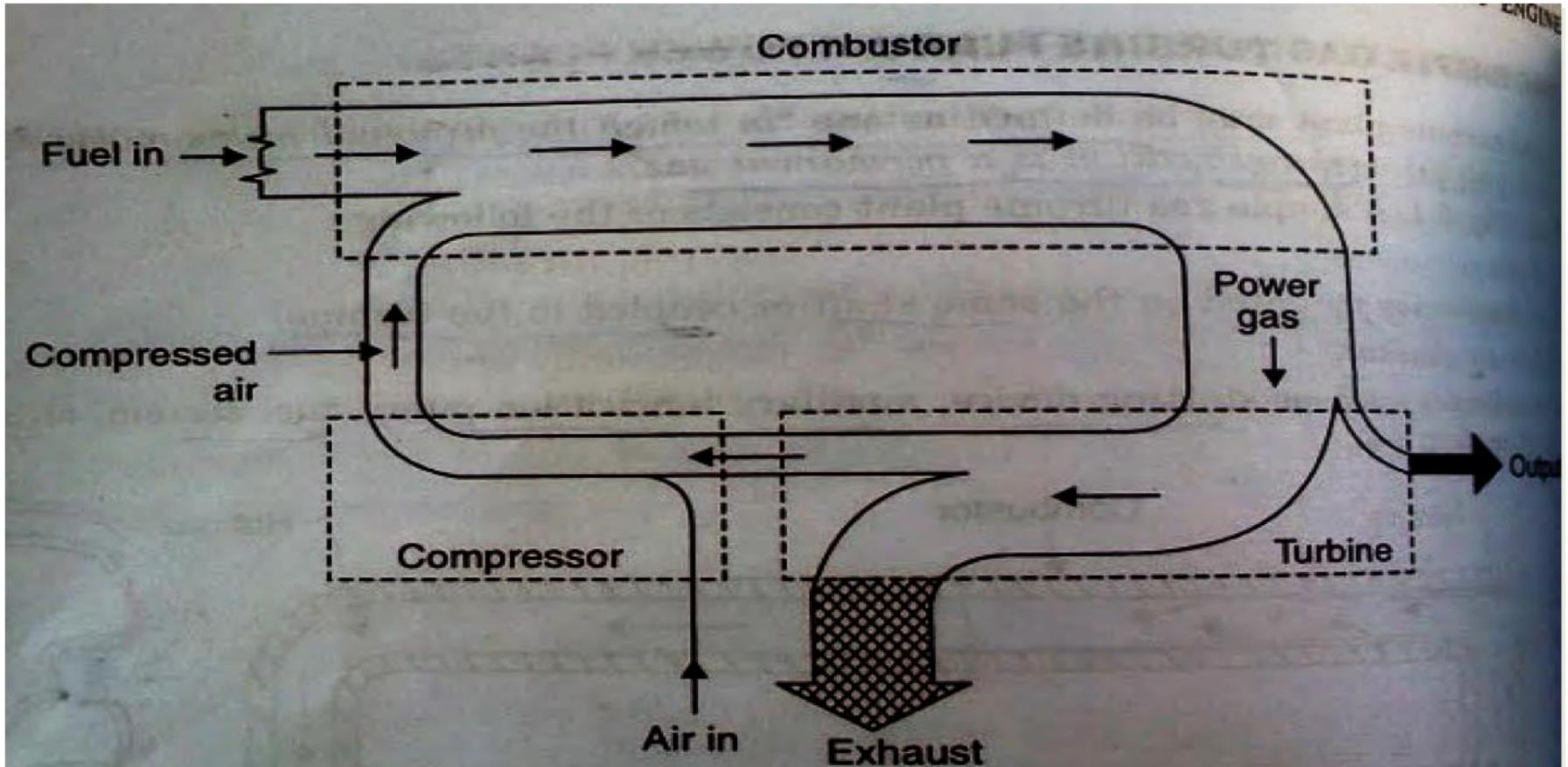
**Fig. 5.2. Energy flow diagram for gas-turbine unit.**
