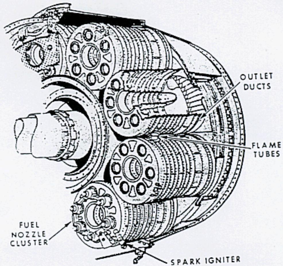
Figure 16-12.—Can-annular-type combustion chamber.
