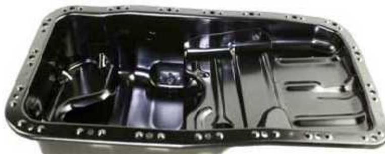
The oil pan serves as a reservoir for the storage, cooling and ventilation of engine lubricating oil.
