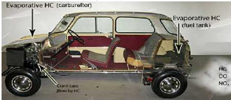
**Emission sources in a gasoline fuelled car.**
